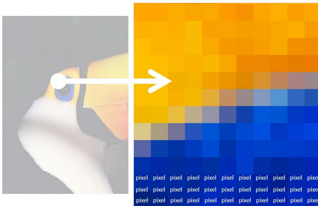
Fig 7. Pixel, the construction block of an Image
